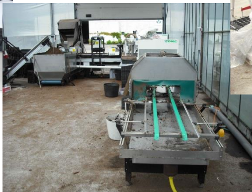
Two semi automatic seeding lines.
