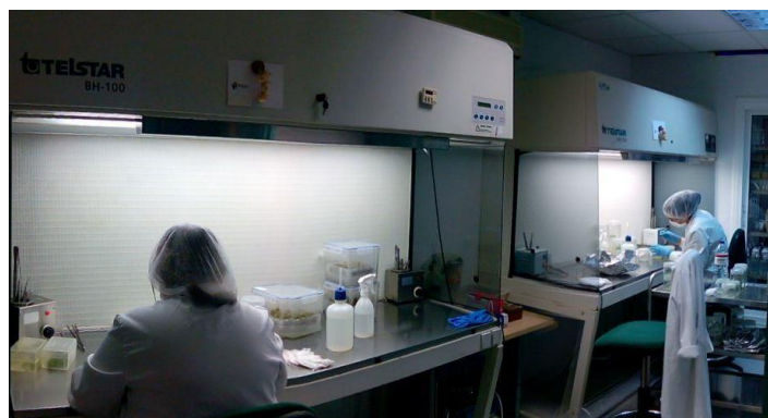
Two laminar flow cabinet
