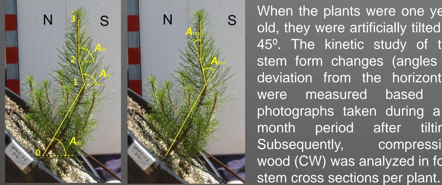
When the plants were one year old, they were artificially tilted at 45°. The kinetic study of the stem form changes (angles of deviation from the horizontal) were measured based on photographs taken during a 6 month period after tilting. Subsequently, compression wood (CW) was analyzed in four
